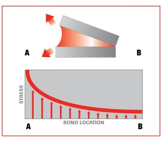
**CLEAVAGE STRESS:** A cleavage stress occurs when rigid substrates are being opened at one end. *NOTE: The stress is concentrated at one end.*
